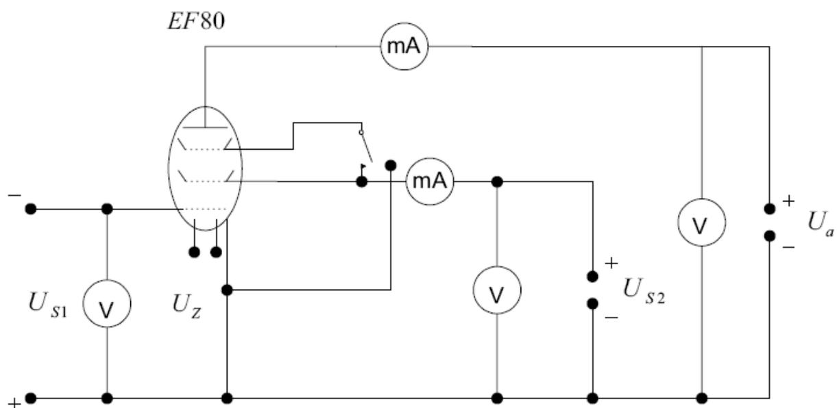
Fig.1: Scheme of the circuit for the measurement of the static characteristics of tetrode and pentode.
